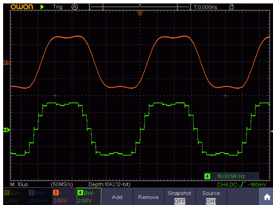
A 10kHz square wave as output by the DAC (green) and after filtering (orange). The (stepped) rise time at 4V p-p is close to 10uS.
