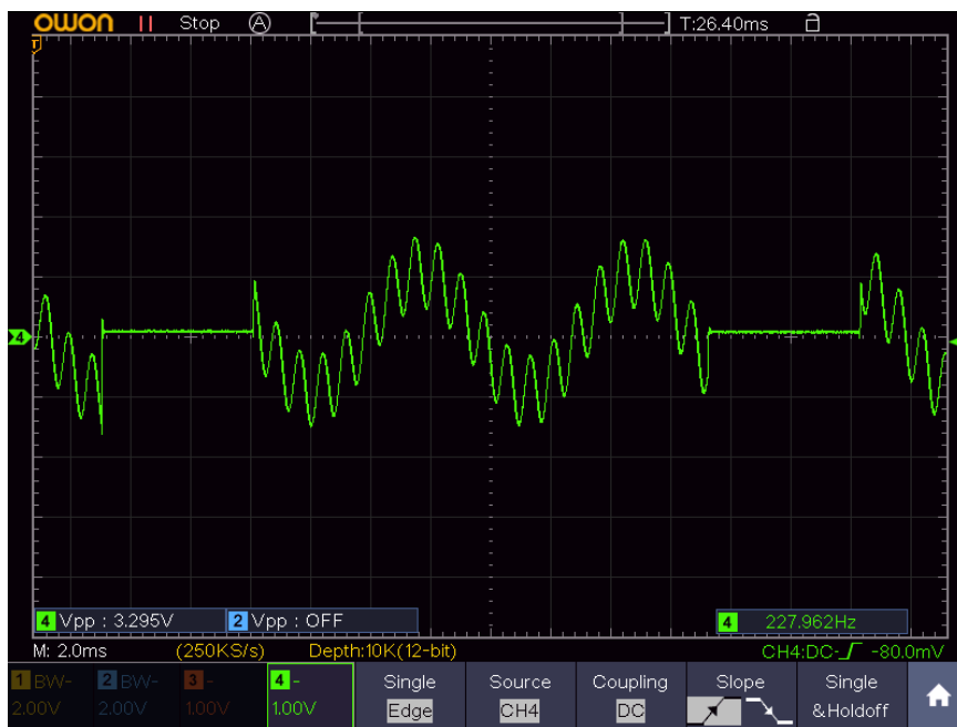
A 150/1500 Hz IMD signal with a 15mS on / 5mS off burst.
